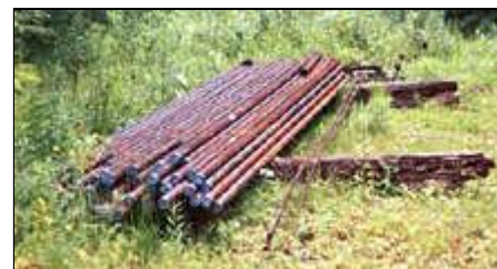
Pulled 2" pipe at a recently plugged and abandoned oil well. This is the type of equipment sampled for NORM
